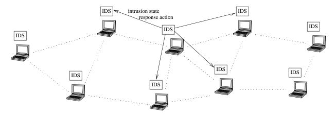
Figure 1. The IDS Architecture for Wireless Ad-Hoc Network
